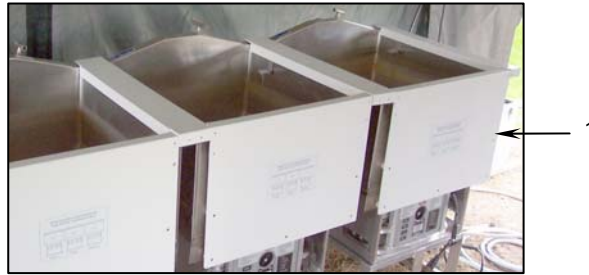
Figure 27. Sink Heat Shield Installation.
