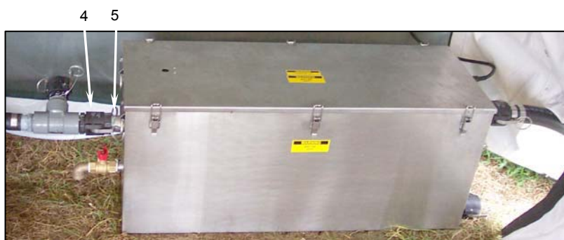
Figure 3. Emptying Water from Grease Separator without the Pump and Bypassing the Pump.
